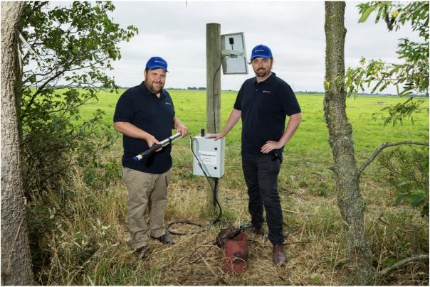
Figure 2: An installation of a HydroMetrics GW50PC on a New Zealand farm to monitor shallow groundwater nitrate levels.
